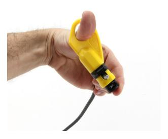
5. Twist the wire braid to draw it back from the edge of the white insulation. Remove any strands of the wire braid that are touching the center copper wire.
