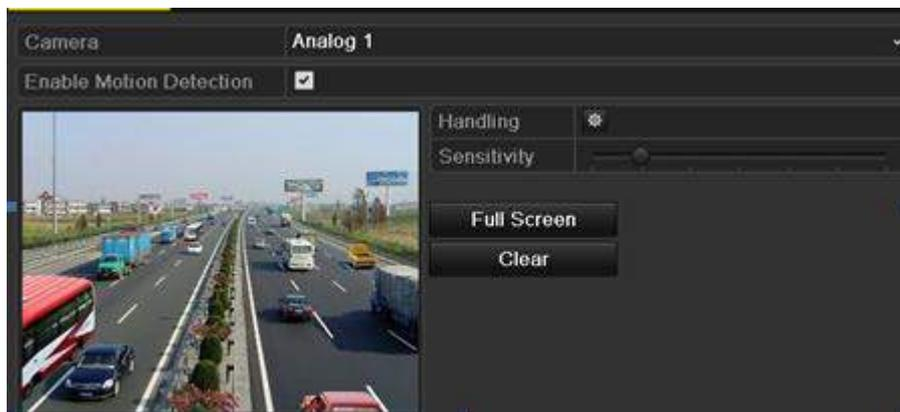
Figure 8. 1 Motion Detection Setup Interface
