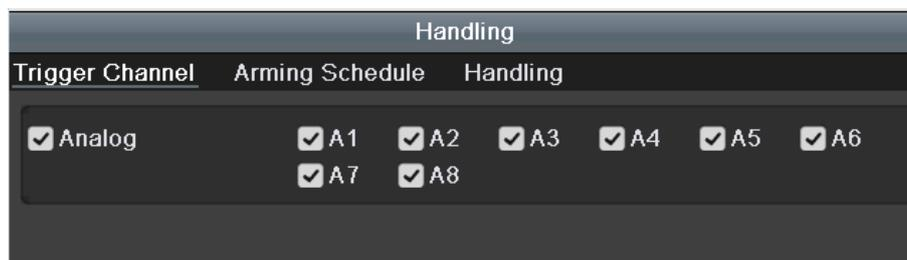
Figure 8. 3 Set Trigger Camera of Motion Detection
